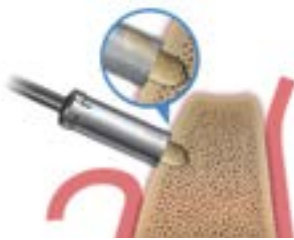
Harvest drill & stopper Bone collection in the buccal side of ridge: 50~200rpm / 30~50N-cm
